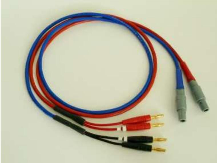
Figure 20. Kelvin Test Leads type "A".
