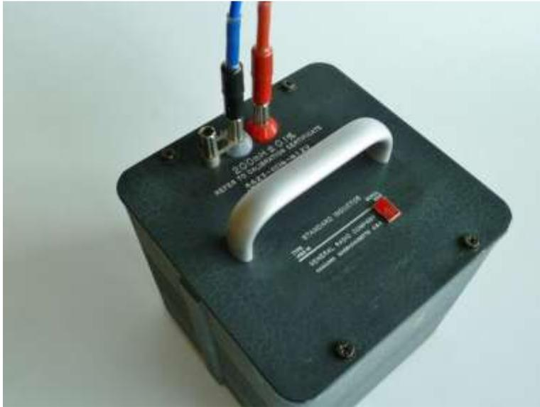
**Figure 6. Connection to Standard Inductor with test leads type “B”.**
