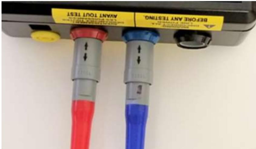
Figure 1. Connection to Instrument with test leads type “A”.
