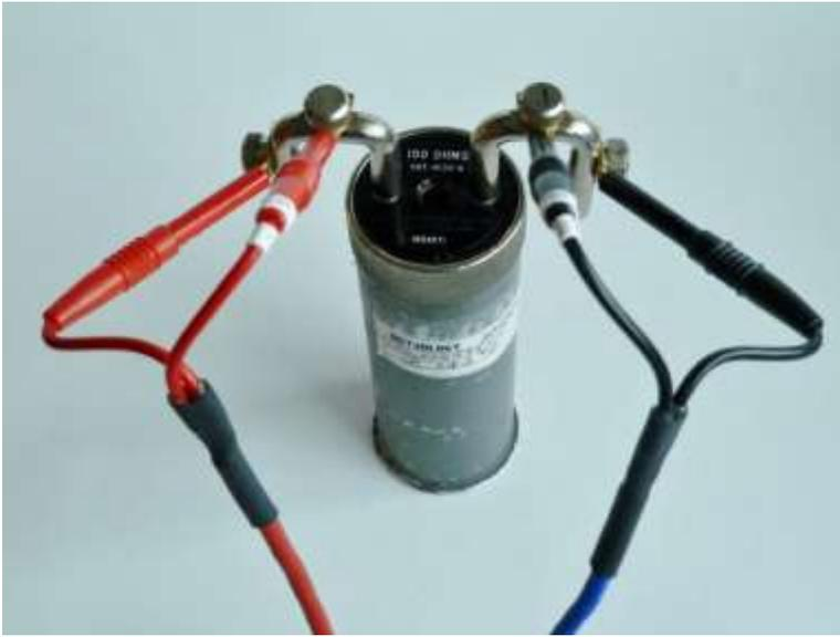
**Figure 3. Example #2: Connection to Standard Resistance with Kelvin test leads type “A”**
