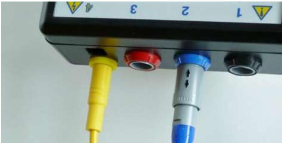
Figure 74. Connection to Instrument with blue test lead type “B” and yellow safety test lead.
