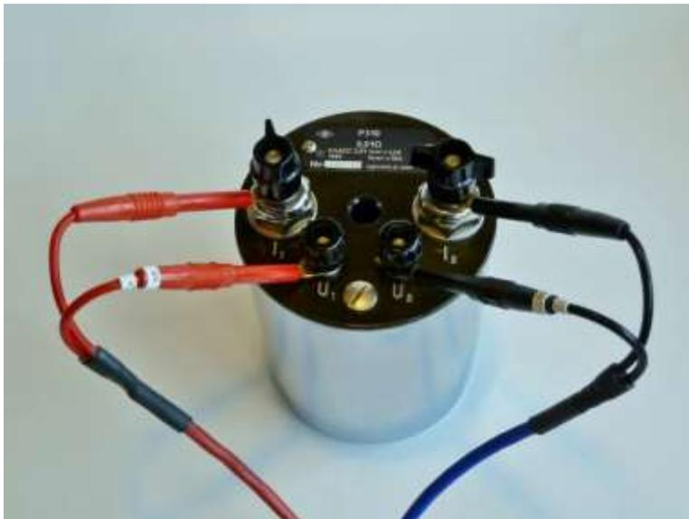
Figure 2. Example #1: Connection to Standard Resistor with Kelvin test leads type “A” and banana plug to open spade lug adaptors. (Note: Sense plugs marked with “S+”=HI and “S-”=LO)
