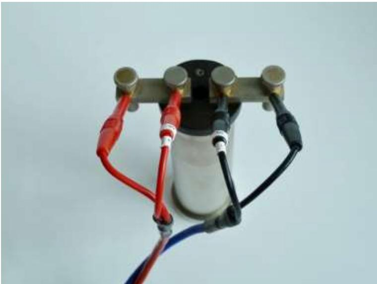
**Figure 4. Example #3: Connection to Standard Resistance with Kelvin test leads type “A”**
