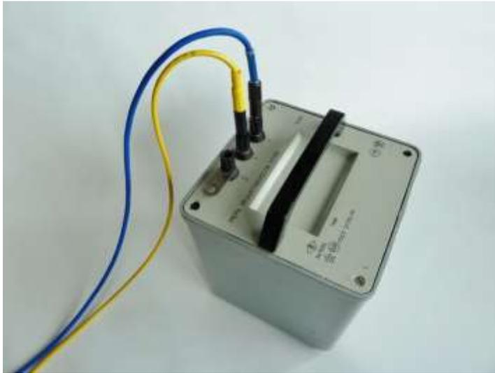
**Figure 85. Connection to  $\geq 1\text{M}\Omega$  Standard Resistor with blue test lead type “B” and yellow safety lead with open banana plug adaptor. (Note: GND connection not used)**
